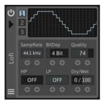
Lofi effect (Bit Crusher + Re-sampler) **Mode(1, 2, 3)** Selects the mode of bit crusher **Sample Rate** Sets the sampling rate of re-sampler **Bit Depth** Sets the bit depth of bit crusher
