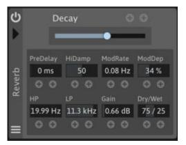
Reverb effect. **Decay** Sets the decay time **Decay** Sets the time of pre delay **Mod Rate** Sets the modulation speed
