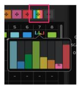
Selecting the Rainbow Block will trigger a random SEQ/ARP block defined by the trigger probability values. You can adjust the probability values of the individual SEQ/ARP Blocks by clicking a BLOCK step where the rainbow block is assigned.
